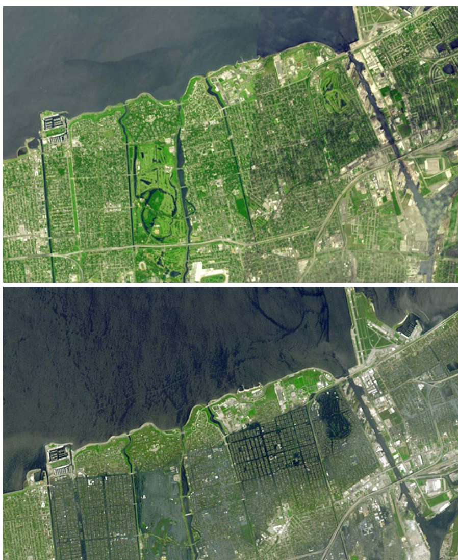
Figure 14: Hurricane Katrina flooded New Orleans, USA (before and after). These two images from NASA's Terra satellite show the affected areas. The top image is from 2000 and the bottom image is from 2005. The flooded parts of the city that are still under water appear dark blue and areas that have dried out appear light blue gray. On the left side of the image, the failed 17th Street canal marks a sharp boundary between flooded city to the east and dry land to the west. The images cover an area of 10.4 x 7.1 kilometres.
